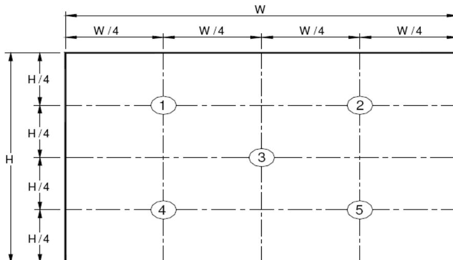
Center Luminance of white is defined as luminance values of center 5 points across the LCD surface. Luminance shall be measured with all pixels in the view field set first to white. This measurement shall be taken at the locations shown in FIGURE 2 for a total of the measurements per display.
